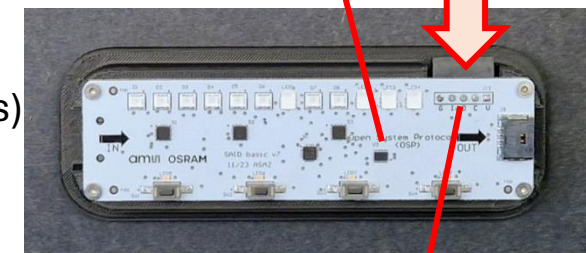
Connector for external EEPROMs
