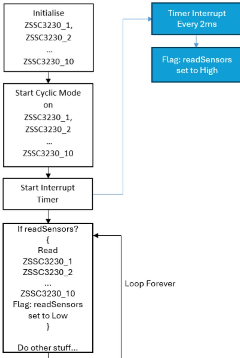
This system will interrupt the infinite loop every 2ms to read 10 ZSSC3230 sensors consecutively. Theoretically, at an I2C clock speed of 400kHz, this should take 1.175ms, leaving time for other calculations or communications. Inside the infinite loop, you could take the data from all the ZSSC3230 sensors, write it to a buffer and transfer it over Bluetooth to a phone.
