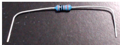
Figure 12: Bend the resistor's leads about 1cm from the ends.
