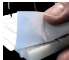
(b) Confirming that the corners of the template are aligned with the corners of the breadboard.
