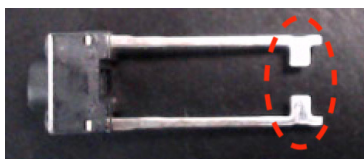
Figure 23: Some momentary pushbuttons have metal tabs on their leads.
