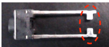
Figure 25: Some momentary pushbuttons have metal tabs on their leads.
