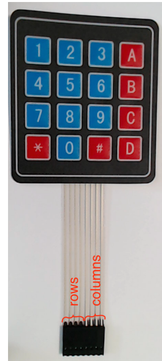
Figure 20: The numeric keypad's header has four row pins and four column pins.
