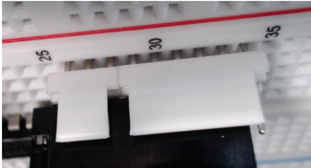
(a) The matrix keypad's connector, with the male-male header strip, just before being inserted into the breadboard. Note the excess header strip's excess pin to the right of the column pins, in contact point j34.
